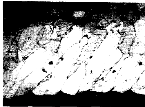
Fig. 8. Complete cross section of 0.04wt.%Ca–0.95wt.%Sn alloy cast on the Cominco Multi Alloy Caster and deformed by stretching. (Note: deformation at grain boundaries and serrated surface; magnification \times 320 .)
