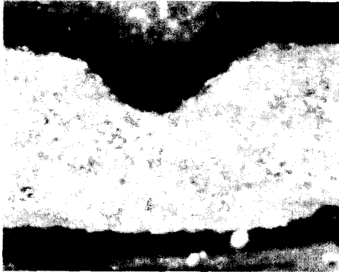
Fig. 20. Grain structure of Wirtz Con Roll Pb–0.06wt.%Ca–1.0wt.%Sn alloy after 2600 hot J240 cycles. (Note: uniform corrosion product and no evidence of corrosion penetration; polarized light; magnification \times 320 .)
